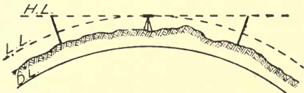
FIG. 125.—Corrections equal when distances equal.
